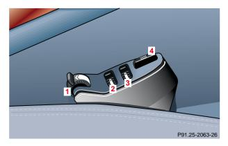
Some models may be equipped with multicontour seats. These seats have movable seat cushions, and inflatable air cushions built into the backrest to provide additional lumbar and side support. We recommend to adjust the multicontour seat in the following order:
